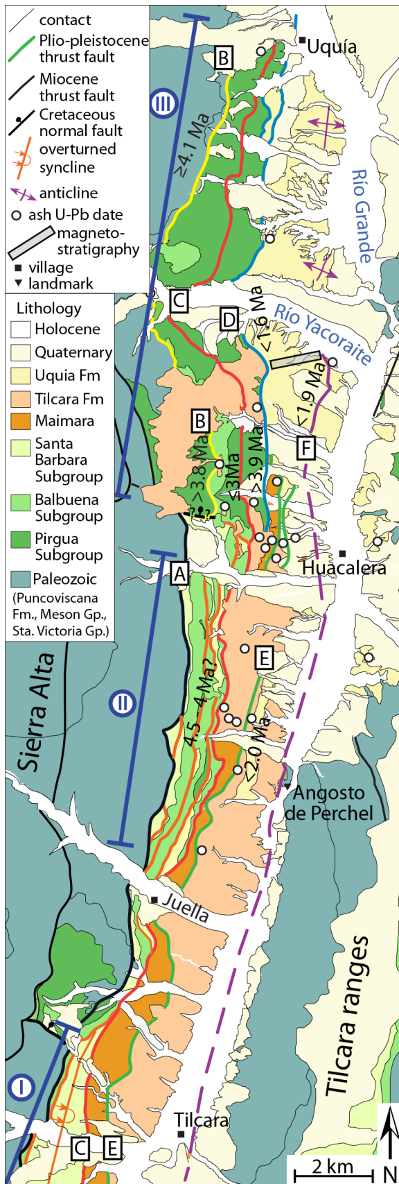
Figure 7. Simplified map of faults in the Humahuaca basin. Fault colors: yellow = Fault B, red = Fault C, orange = faults in hanging wall of Fault C, blue = Fault D, green = Fault E, purple = Fault F. Segments of faults on western margin of basin are labeled (I, II, III) on the left. White circles indicate sample locations that provide constraints on timing of deformation. Age labels on faults indicate when that fault was active: > means fault was not active after that time; < means the fault was active sometime after that time (but could have been active before then as well).
