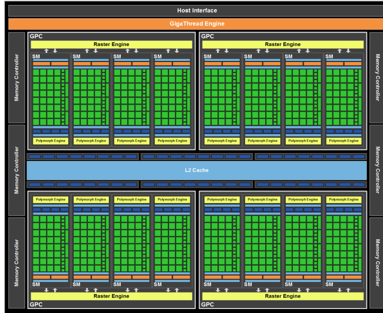
Figure 3.1: Block diagram of an Nvidia GF100 GPU, whose Fermi architecture is similar to the GPUs present on Knot and Braid. The device is organized into 16 “streaming multiprocessors” or SMs, each of which contains 32 cores for standard arithmetic instructions. Figure adapted from http://images.anandtech.com/reviews/video/NVIDIA/GF100/GF100.png .
