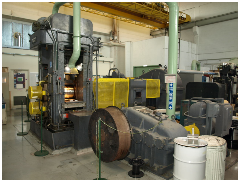
Figure 3.2: Waterbury Farrel rolling mill at the LANL Sigma Complex used for ARB processing.
