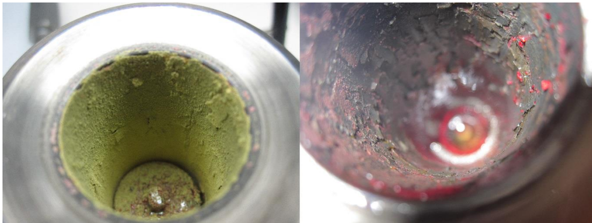
Figure 11. Inconel 625 reactor body after a run with \text{NH}_4\text{Cl} mineralizer. Yellow powder that was highly soluble in water was often found (left) as were red crystallites (right). The red crystallites were water soluble but took much longer to dissolve than the yellow powder. Note also the scaling and spalling of the walls on the right.
