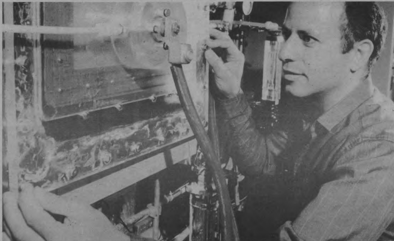
Dr. Robert Homsy, a chemical engineer at Lawrence Livermore Lab, demonstrates an aluminum-air fuel cell being developed as a refuelable power source for electric
