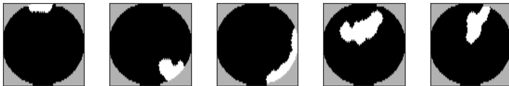
Figure 4.11: Binary pattern examples. Note that the regions outside of a wafer map should be in black (zero values) and are shown as gray regions for better visualization.
