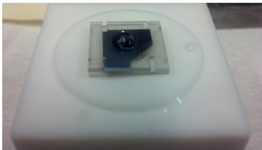
Figure S93 – Custom Teflon chamber used during transport experiments as outlined in Chapter 5.
