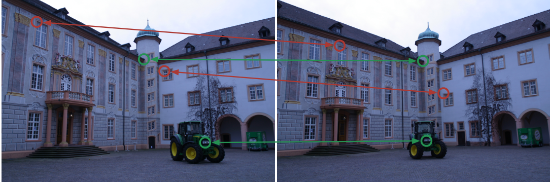
Figure 4.3: The image correspondence problem aims to find pixel locations on a query image (left) and a reference image (right) depicting the same 3D point from the scene. The common way to estimate a putative set of correspondences is by means of the nearest neighbor classifier. First, a set of features or keypoints (depicted as circles) in both images are detected. Subsequently, for every keypoint a descriptor, which is a representation encoding photometrical information of the surrounding pixel neighborhood, is computed. Finally, the nearest neighbor classifier finds the most similar reference descriptor for every query descriptor to establish a putative correspondence. This process is far from perfect and produces correct and incorrect putative correspondences (shown in green and red, respectively).
