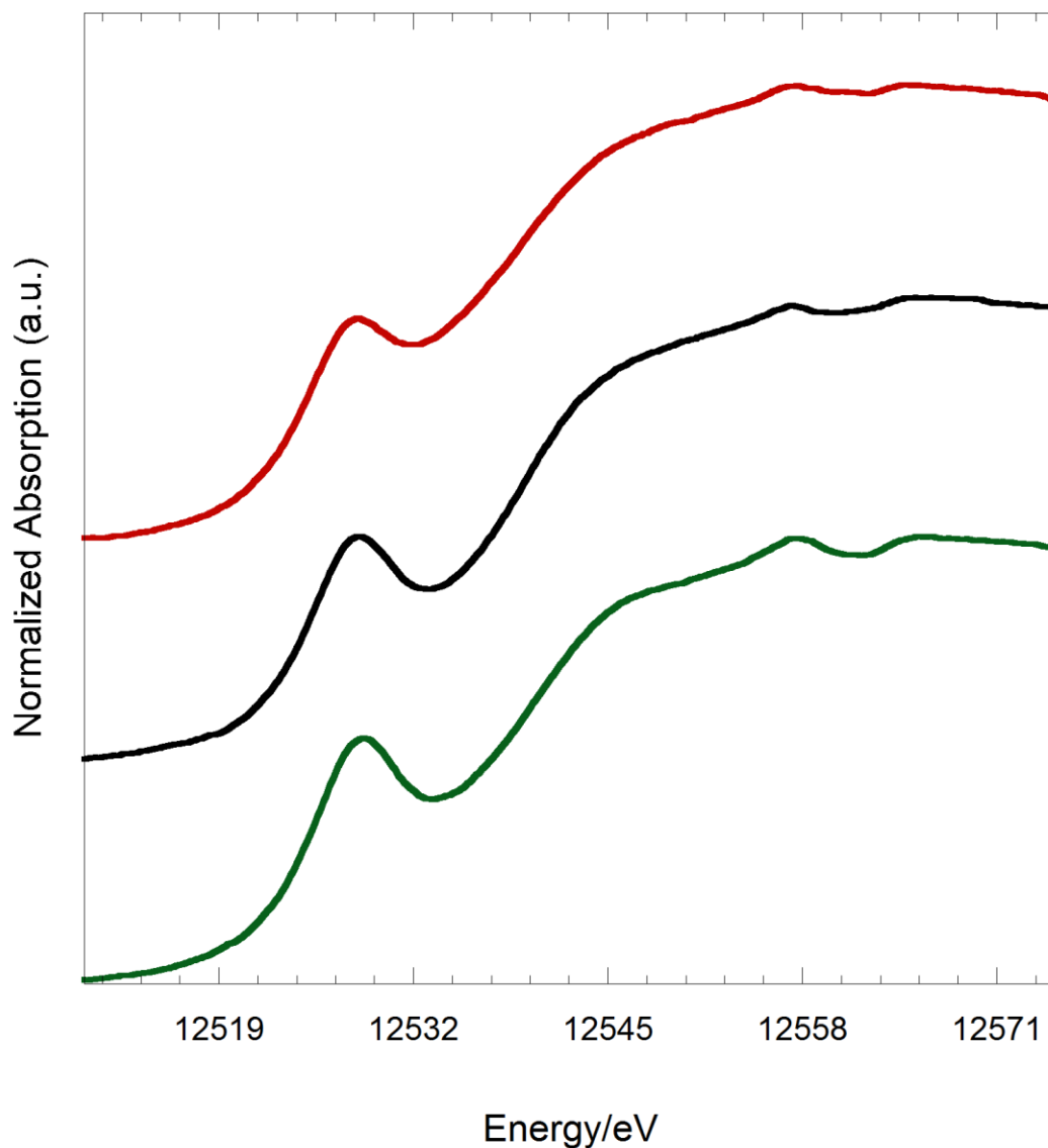
Figure D.4: X-ray Absorption Spectra at Re L_1 edge for MTO (green line), MTO on \gamma - \text{Al}_2\text{O}_3 (black line) and MTO on \text{Cl-Al}_2\text{O}_3 (red line). A prominent pre-edge, caused by the dipolar 2s \rightarrow 6p transition, is detected at 12526 eV for all samples revealing a non-centrosymmetric geometry of the Re sites that cause an hybridization of the 5p-6d orbitals. The same pre-edge feature was detected for \text{Re}_2\text{O}_7 and \text{NH}_4\text{ReO}_4 . 2 The position of the edge at 12539 eV for all samples is compatible with the presence of Re(VII). After grafting of MTO both on alumina and chlorinated alumina no substantial differences among were detected in the spectra.
