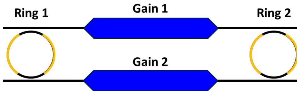
**Figure 6.** Illustration of the Vernier ring laser first iteration.
