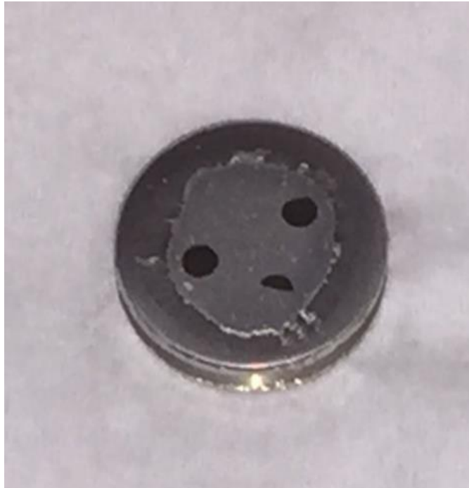
Figure 3.2. Three specimens (LD, LG and CM6) mounted on an SEM stub with Durabond adhesive prior to annealing.
