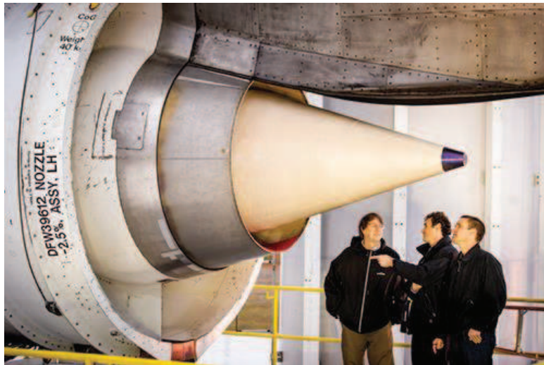
Figure 1.1: Oxide/oxide CMCs in commercial engines: (a) mixer and center body assemblies in General Electric's Passport 20 engine (Eldrid et al., 2001); (b) exhaust nozzle for the Boeing 787 Dreamliner (Wood, 2013).
