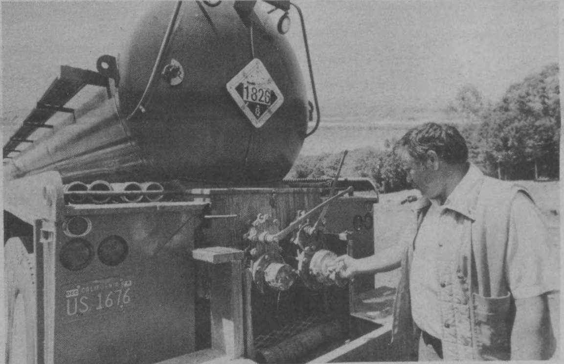
David Lomeli, Highway Superintendent of Cal Trans, points to the charge-discharge pipes where toxic chemicals are loaded and drained from the truck tank. Below, a ten-inch crack in the pipes underneath the truck was caused by the combination of toxic chemicals.
