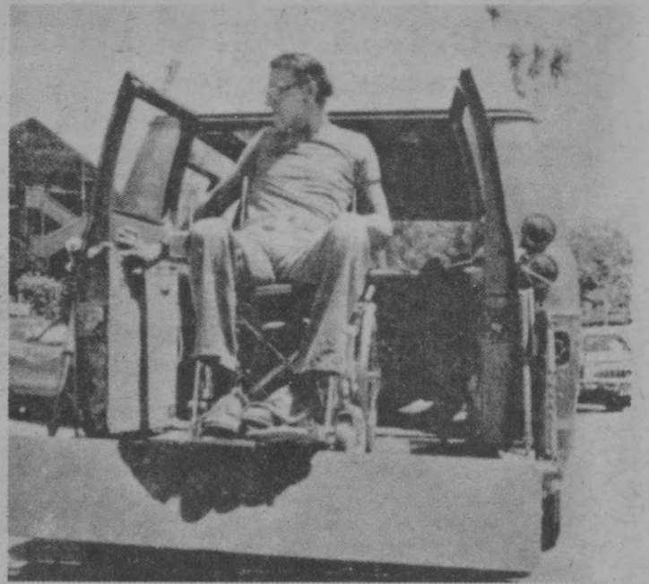
CHAIR LIFTS, like the one shown above, provide a way for some disabled persons to travel unassisted, bridging what used to be a significant barrier.
