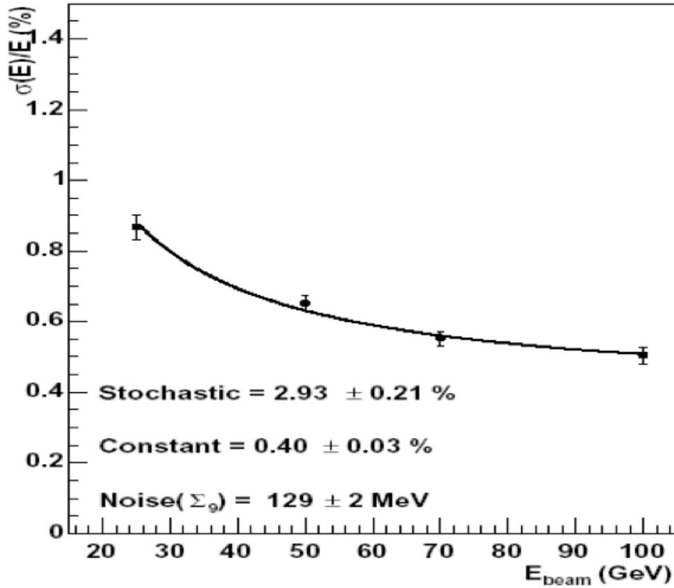
Table 5.2 shows contributions ( anticipated for the ECAL design ) to the stochastic, noise, and constant terms in the total energy resolution as a function of energy in the EB, ECAL Preshower detector and EE. Figure 5.3 shows the energy resolution as a function of energy measured with an electron test beam of known energy.
