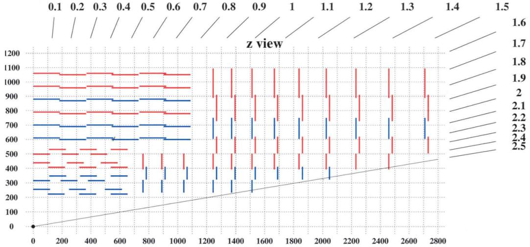
Figure 4.8: CMS Silicon Strip Tracker  $r - \phi$  View. Single-sided modules are shown in red while double-sided ( stereo single-sided ) modules are shown in blue [2].
