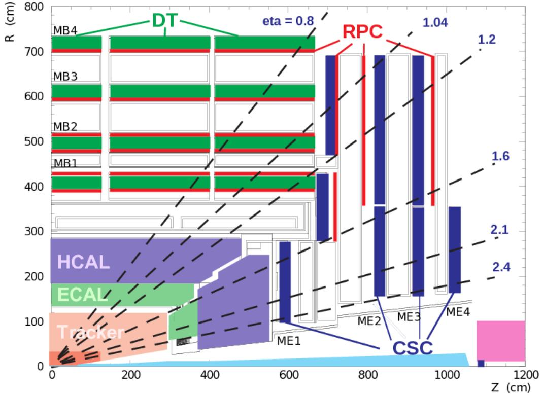
Figure 7.2: Detailed Layout of the CMS Muon System [6].
