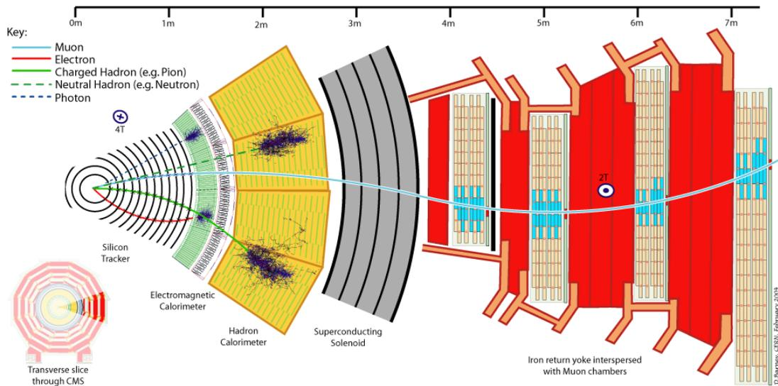
The CMS detector can be described in a cylindrical coordinate system with the collision point at  $r = 0$ ,  $z = 0$ . Figure 2.16 shows a cross section of the CMS detector in the transverse  $r - \phi$  plane. CMS has several subsystems which
