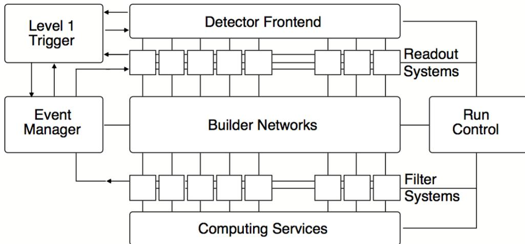
The L1 trigger makes decisions local to the ECAL, HCAL, and Muon subsystems while the HLT makes global decisions after synchronizing L1 information from different subsystems including the Tracker. The L1 trigger is factored into three subsystems: the L1 Calorimeter Trigger, the L1 Muon Trigger, and the L1
