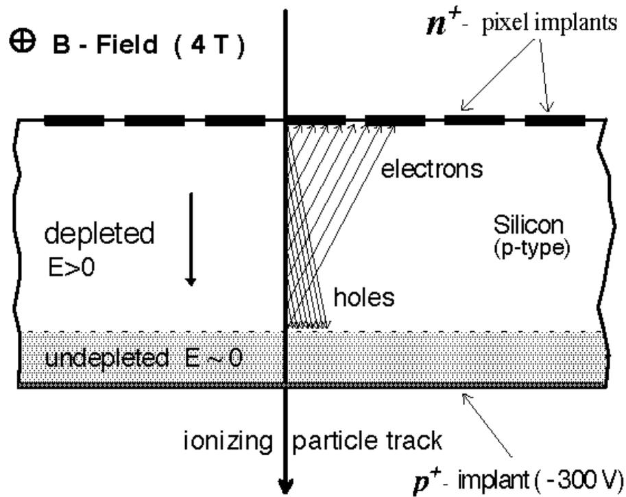
Pixel detectors in a magnetic field are subject to Lorentz drift of charge carriers in the bulk which leads to charge sharing between neighboring pixels. The CMS pixel detectors are designed to exploit charge sharing in order to improve position resolution from  $\sim 35\ \mu\text{m}$  to  $10\ \mu\text{m} - 20\ \mu\text{m}$ . In a  $4\text{ T}$  magnetic field the Lorentz drift angle characteristic of electrons is  $32^\circ$ , which is three times larger than the
