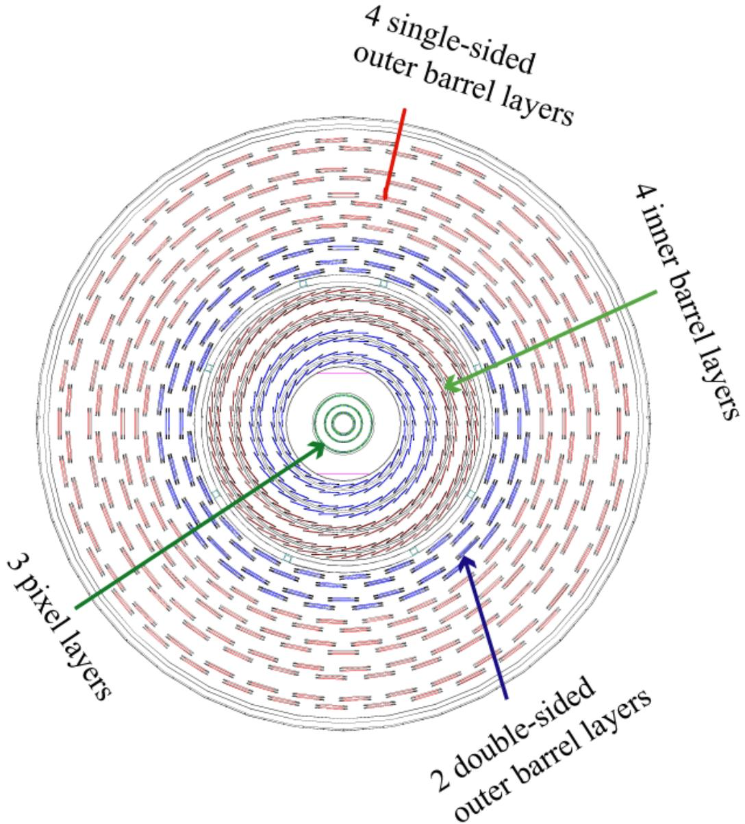
The TIB consists of 4 layers located at radial positions of  $25\text{ cm}$ ,  $34\text{ cm}$ ,  $43\text{ cm}$ , and  $52\text{ cm}$ . The two inner layers of the TIB are double-sided with a strip pitch of  $80\ \mu\text{m}$  while the outer two layers are single-sided with a strip pitch of  $120\ \mu\text{m}$ .
