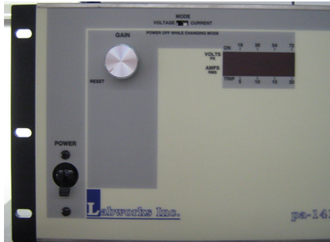
Figure A.3: Front panel of the amplifier with a voltage and current indicator, on/off power switch, and gain knob.
