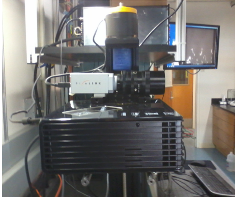
Figure A.12: Seen from the side is the projector and camera supported by a vertical stage.
