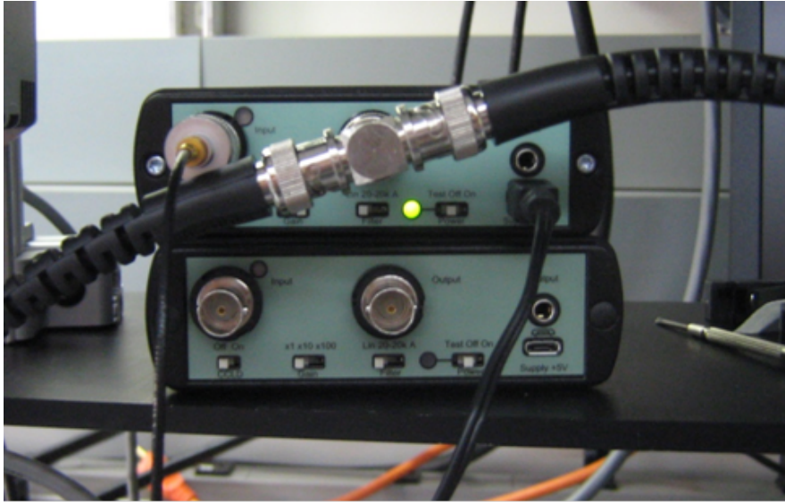
Figure A.6: Two accelerometer signal conditioners with only the top in use. The BNC output is split and sent to the DAQ and oscilloscope.
