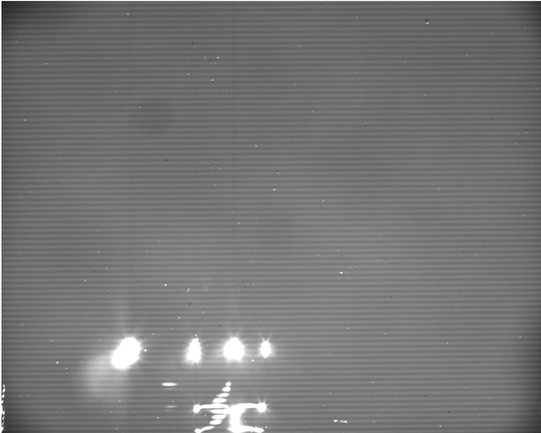
Figure 4.4: An image captured later after the formation of Faraday waves which are not visible. The bright spots at the bottom on the image is the projector filament since once standing waves form with a sufficiently large slope, light is reflected from the projector directly into the camera.
