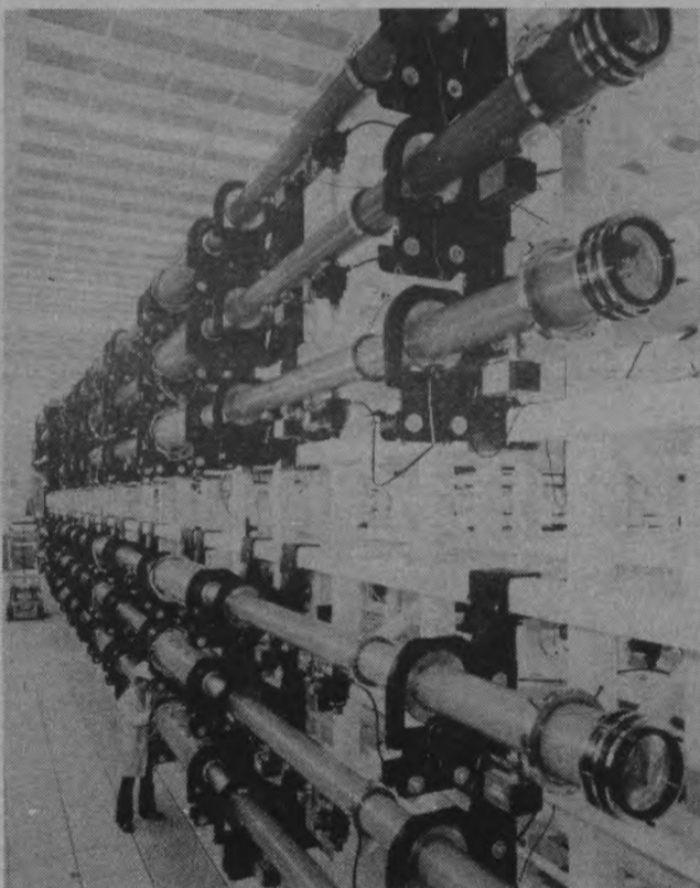
Above right, six of the twenty laser amplifier beams of the Shiva laser. At left, the target chamber of the Shiva where 30 trillion watts of optical power are focused onto fusion fuel located in a target the size of a grain of sand.
