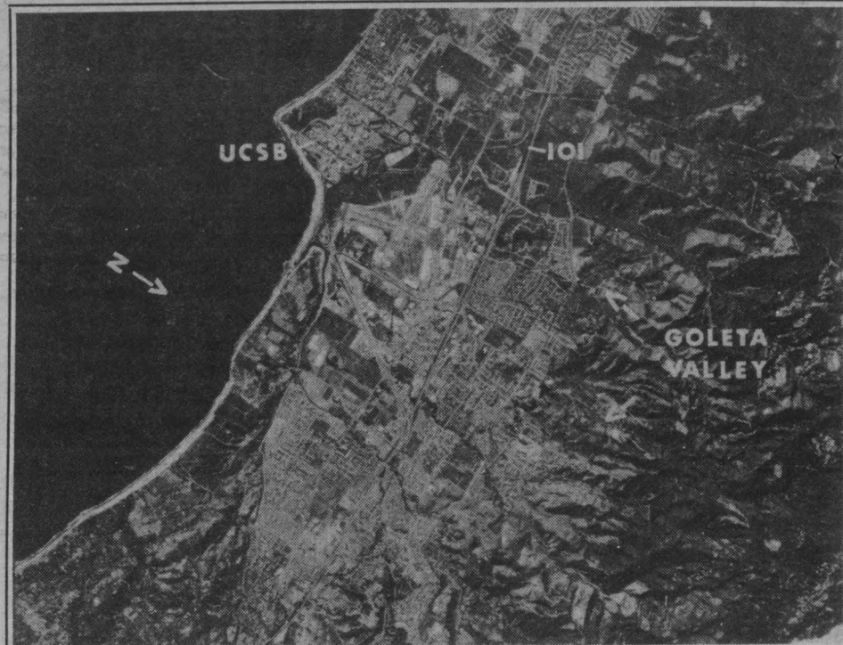
REMOTE SENSING Cars on highway and even white lines in parking lots can be distinguished in this black-and-white copy made from a portion of an infrared Ektachrome aerial photograph of the Goleta Valley taken from 60,000 feet with a six-inch focal length lens in a continuing study of land use changes being carried out by the UCSB Geography Remote Sensing Unit.
