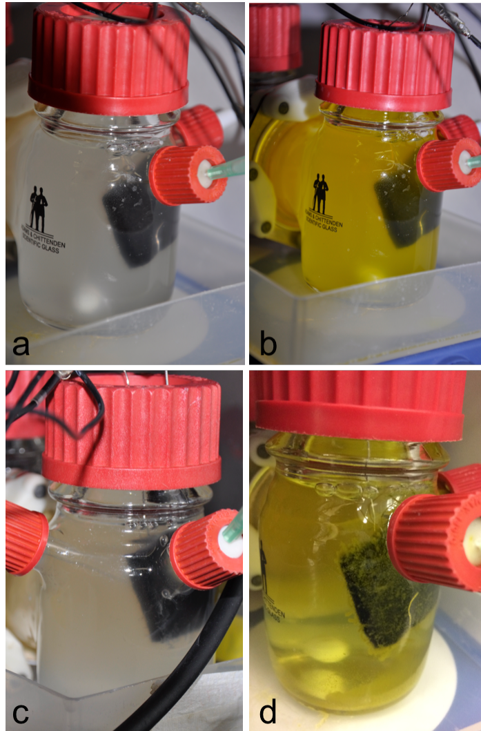
Figure 4.12: Photographs of bioreactors at time of DSSN+ addition ( t = 3.6 h) and at t = 12 h. At t = 3.6 h, bioreactor solutions were visibly turbid at OD_{600nm} = 0.55 \pm 0.04 for all (a) untreated and (b) DSSN+ treated bioreactors. After overnight operation ( t = 12 h) solutions from (c) untreated bioreactors were still visibly turbid, while solutions from (d) DSSN+ modified bioreactors were visibly less turbid with cell mass adhered to electrodes.
