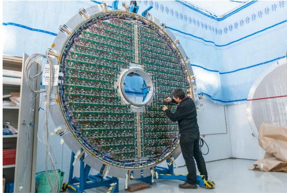
Figure 3.25: The preshower detector, to be installed in front of the crystals in the electromagnetic calorimeter endcap. Photo: CERN.
