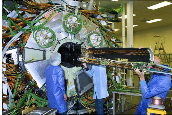
Figure 3.12: Installing the pixel detector into the center of the tracker assembly. Photos: CERN.
