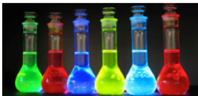
Figure 1.4 Volumetric flasks containing various organic semiconductors for light-emitting diode applications. This image is copyright Cambridge Display Technologies.
