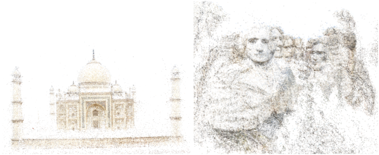
Figure 1.1: Structure-from-Motion is able to recover a 3D models of world landmarks such as the Taj Mahal and Mount Rushmore. Viewers are able to freely explore these 3D models to observe the scene from any angle and position to gain a better understanding of the scale and structure. This enables viewers to observe the scene from novel viewpoints that may not be easily accessible in the real world.
