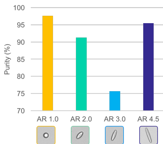
(a) Purity for each particle type after performing the 2-D sort
