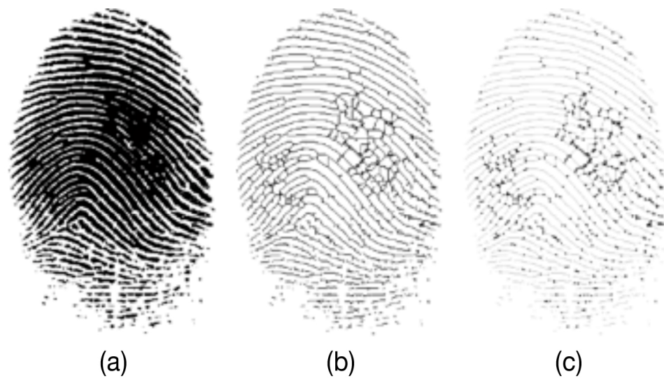
Figure 5.3.1: Visual feature extraction of a fingerprint sample from FVC2004 dataset. Image skeletonization and minutiae analysis are applied to find singular points on the fingerprint.
