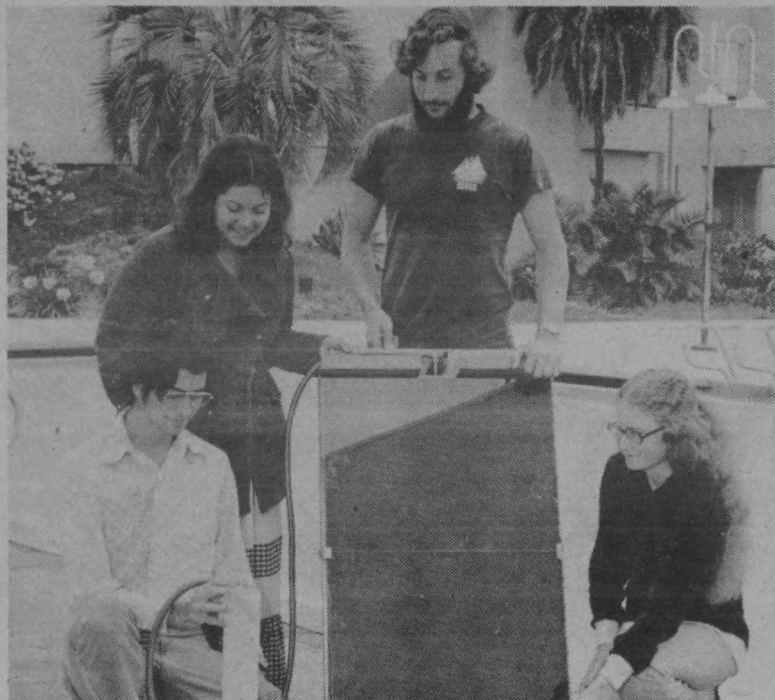
SUN POWER — Measuring flow rate of solar heater which they designed and built for a freshman seminar in chemical and nuclear engineering are UCSB students (from left) Peter Lombrozo, Valery Forestiere, Samuel Louke and Jennifer Robart. Students are comparing computer projections with actual performance of heater. Wilfred Swalling photo
