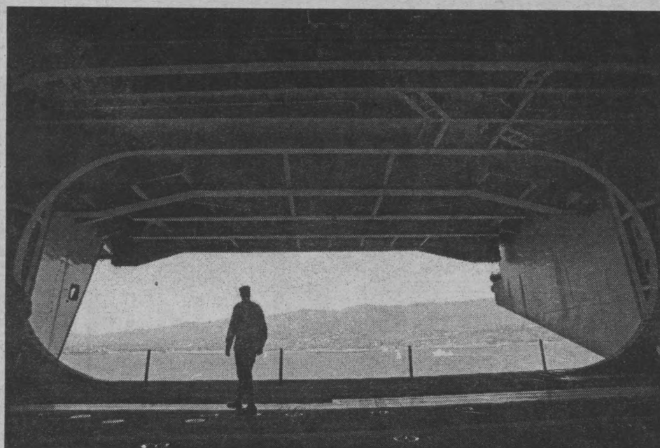
A USS Abraham Lincoln crew member stands before enormous elevator cargo doors large enough to enable both aircraft and personnel to be lifted from the hangar to the flight deck.
