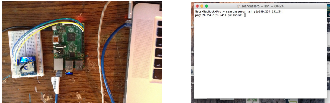
Figure 28. Headless Raspberry Pi ssh connection via Laptop (left) SSH terminal window (right)
