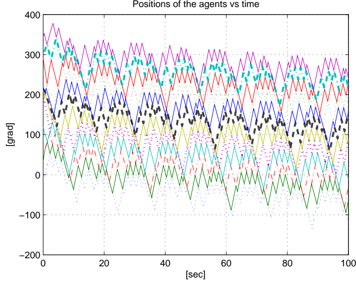
Figure 5.8: This figure shows \theta_i vs time, obtained by implementing the SIS ALGORITHM with n = 12 beads, the beads are randomly positioned on \mathbb{S}^1 , v_i(0) uniformly distributed in ]0, 1[ , d_1(0) = d_4(0) = d_6(0) = d_7(0) = d_8(0) = d_9(0) = d_{10}(0) = -1 , and f = 0.87 . The positions of the beads 2, 4, 6, 8, 10, 12 are represented by solid lines, while the dash line, dash-dot line, point line, and thicker dash line represent the positions of beads 1, 3, 5, 7, 9, 11.
