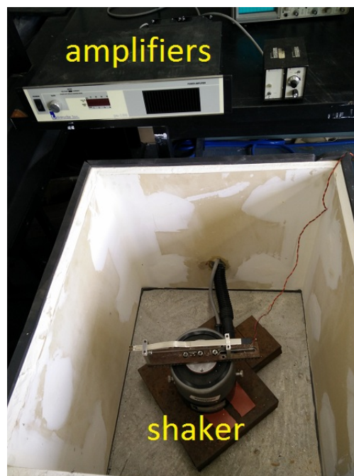
Figure 3.3: The shaker mounted on its vibration isolation platform and surrounded by a sound reducing enclosure. The amplifiers can be seen in the upper portion of the picture, with the shaker amplifier on the left and the piezoelectric charge amplifier on the right.
