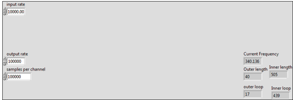
Figure B.6: The control panel for the raw data collection program. Here we can control the sampling rates of both the input and the output, and we can control how many samples are used to generate the signals. Feedback from the program comes as the current frequency, and some tallies to keep track of where in the program it is at.
