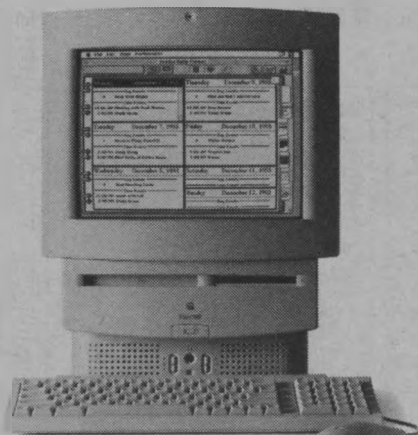
Macintosh LC 520 5/80, internal AppleCD™ 300i CD-ROM Drive, Apple Keyboard II and mouse.
