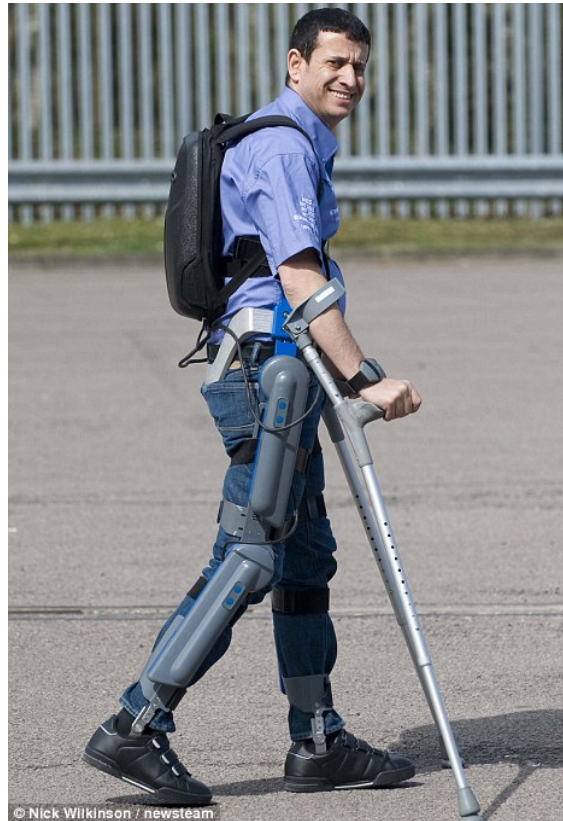
Figure 1.6: The Rewalk system shown above weighs 23.3kg and can cost in the range of $69k to $85k. The cost is a significant burden to users as of yet health insurance does not cover the use of this device.
