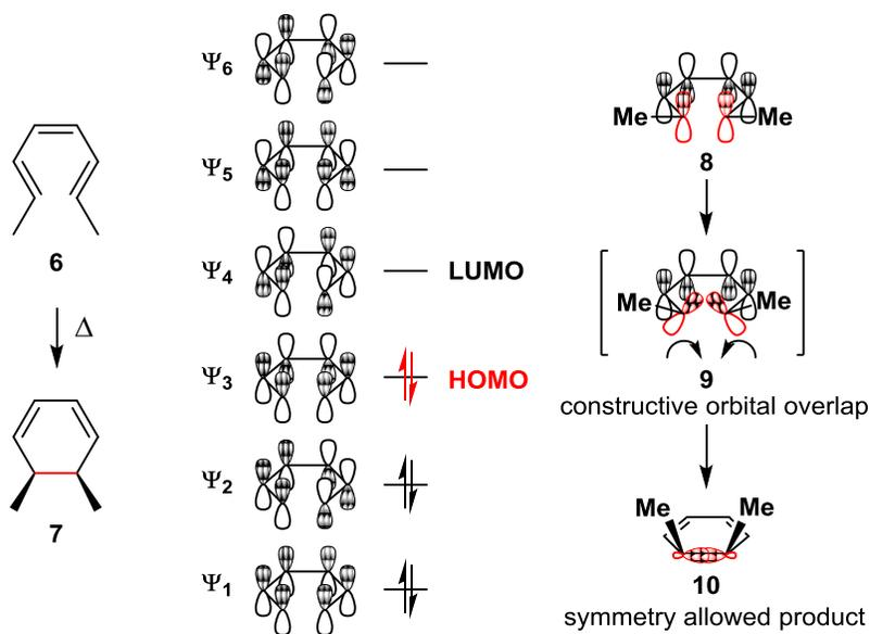
**Figure 2.** Molecular orbital diagram for a thermally promoted 6 $\pi$  electron disrotatory electrocyclozation.
