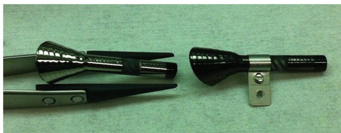
Figure B.3: Schematic of the Stanford Research Systems Model RGA200 residual gas analyzer's detector assembly (upper) and photograph (lower) of new (left) and damaged (right) continuous dynode electron multiplier.
