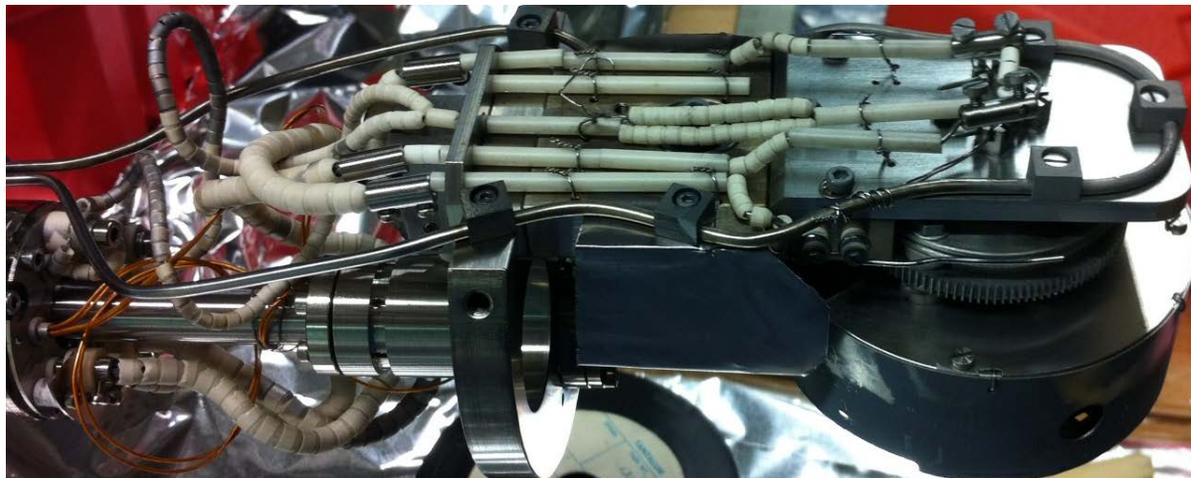
Figure B.2: Rear/Side view of the substrate manipulator near the continuous azimuthal rotation mechanism.
