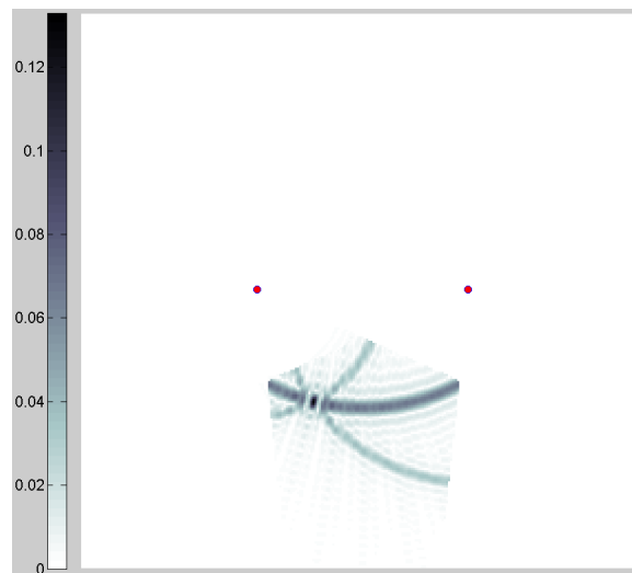
(b) Reconstruction showing a limited applicable area as a result of binary beamspread.
