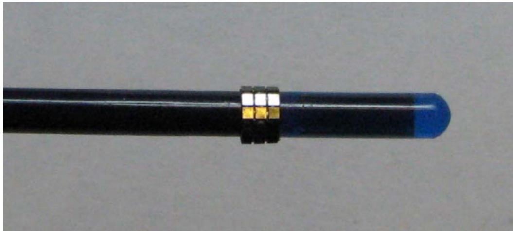
(a) Conformal array wrapped around a 9F (3 mm diameter) commercial intracardiac ultrasound catheter.
