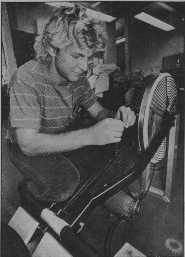
Senior Ted Miller, left, assembles the chain connecting the fly wheel to the generator of the project he and his partners are constructing — the Human Generator. The machine utilizes a rowing mechanism and a fly wheel to transform human energy into kinetic energy, then uses a generator to change the kinetic energy into electric energy. This power, equal to approximately 200 watts, can be returned to the electric company or sent through an appliance.
