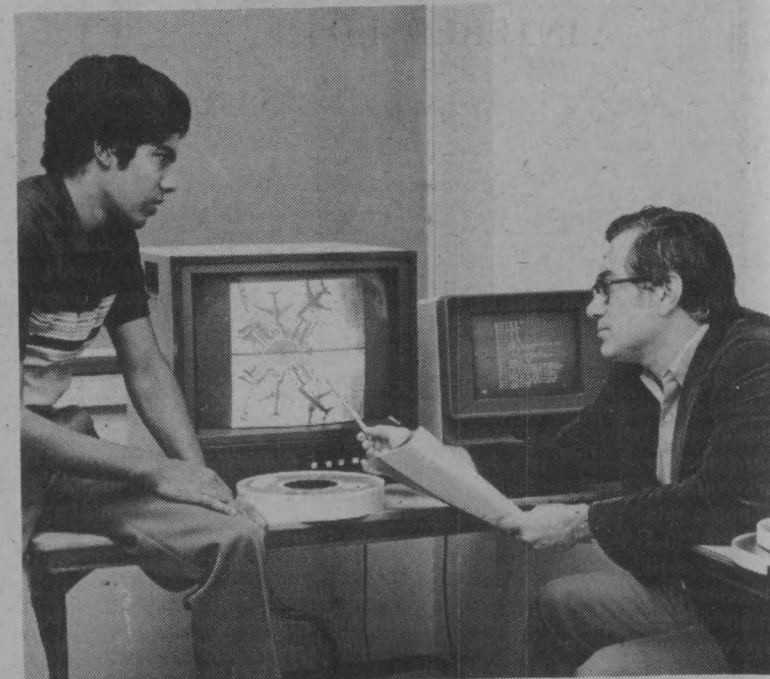
Which is the original picture of Los Angeles International Airport scene and which is the copy processed using vector quantization? Allen Gersho, professor of electrical and computer engineering, right, and Bhaskar Ramamurthi, graduate student and research assistant in the department, compare the quality of the two images. Original is on the top of the screen, while copy is on the bottom.
