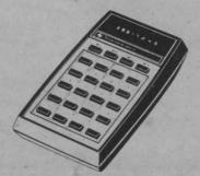
Everything the TI-1200 has—plus. Full function memory: add, subtract, recall or clear with a single keystroke. Also, a change sign key. Replaceable battery. Optional adapter available.
