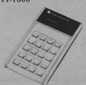
Super slim. High-styled. Four functions. Percent key. Automatic constant. 8-digit display is easy on the eyes. Use it 3 to 5 hours before recharging. AC adapter/charger and carrying case.
