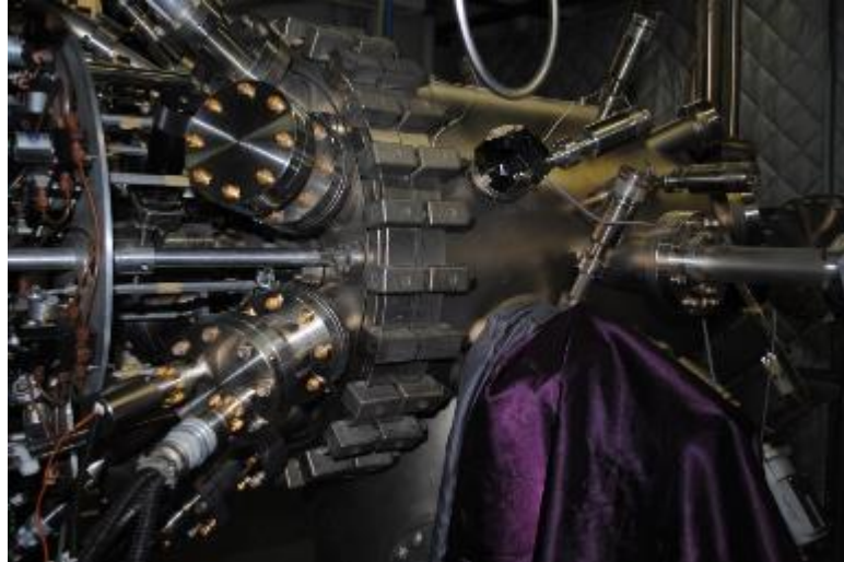
Figure 6 -- The Nitride Gen II growth chamber as seen from the front right of the source flanges.
